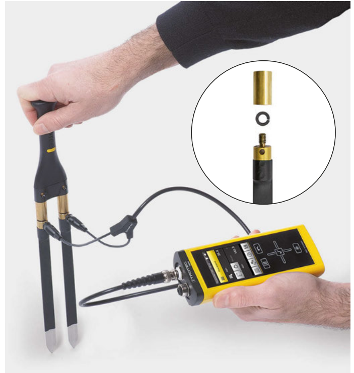
With the TS 60 adapter set (19) all MultiMeasure electrodes can be directly attached to the hand electrode TS 60 (9). For this purpose, the adapters are threaded on both sides and are simply screwed in between the electrode head and the retainer tip of the hand electrode by means of a clamping ring.
