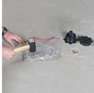
Step 2: Comminution of the sample material so that the entire test material has a grain size not larger than 8 mm.
